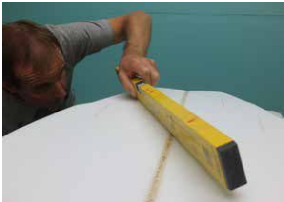
A straight edge reveals more than the eye can detect as the curves, flats and edges blend, meet and morph along the length of this Modern Quad shape.
