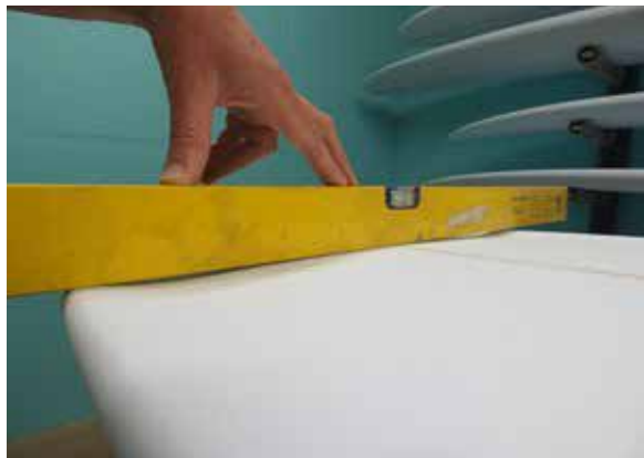
Rail tuck meets rail edge meets concaved curve blending into the bottom curve at the stringer line. The far right side of the level reveals a few millimetres of Vee is also present.
